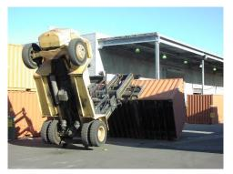
**OSHA Standard 1910.178** covers the requirements for forklifts of all types including rough terrain forklifts, telescoping or boom forklifts, and industrial forklifts. For other mechanized equipment such as loaders. and excavators look to OSHA Standard 1926.600.
