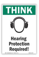
**OSHA Standard 1926.52(b)** When employees are subjected to sound levels exceeding those in Table D-2 of this section, feasible administrative or engineering controls shall be utilized. If such controls fail to reduce sound levels within the levels of the table, **personal protective equipment** as required in Subpart E, **shall be provided** and used to reduce sound levels within the levels of the table.
