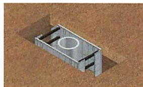
CORNER END PLATES HELP PREVENT LOOSE MATERIAL FROM RUNNING INTO THE END OF THE SHIELD. SOIL AT ENDS SHOULD BE SLOPED ACCORDING TO MANUFACTURER'S TABULATED DATA
