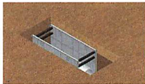
*CENTER SHIELD OVER WORK AREA *LAY SOIL AT ENDS BACK ACCORDING TO MANUFACTURER'S TABULATED DATA OR USE MANUFACTURER'S DESIGNED PLATES TO PROTECT FROM CAVE-INS
